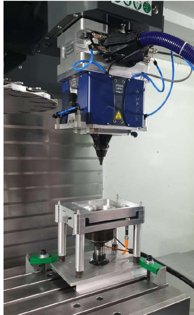
2 The FSW head takes the milling add-on thanks to automatic pressure system
