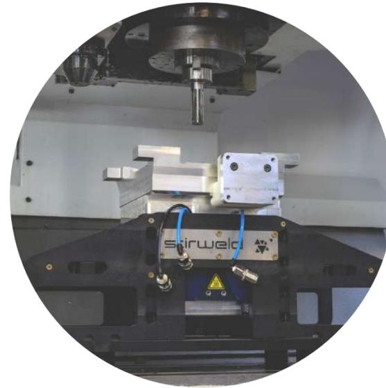
1 Using the head box, move the whole unit onto the machine table.
