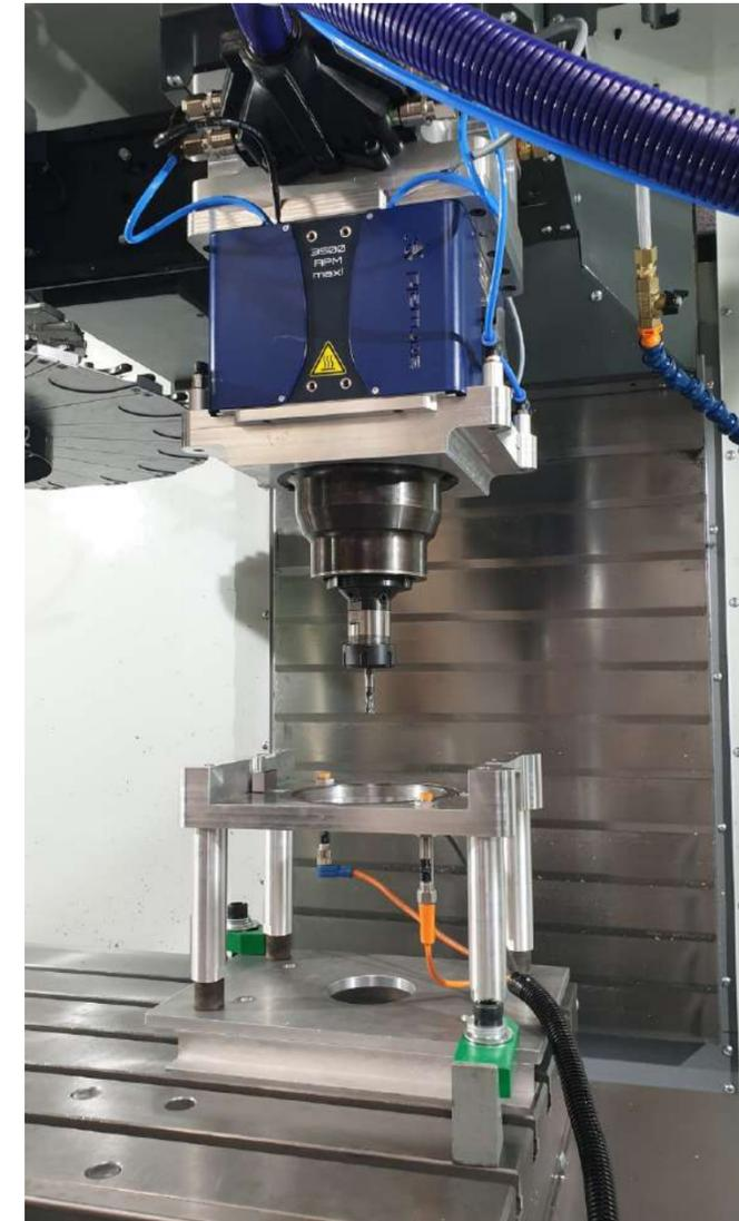
3 The FSW head is ready for milling
