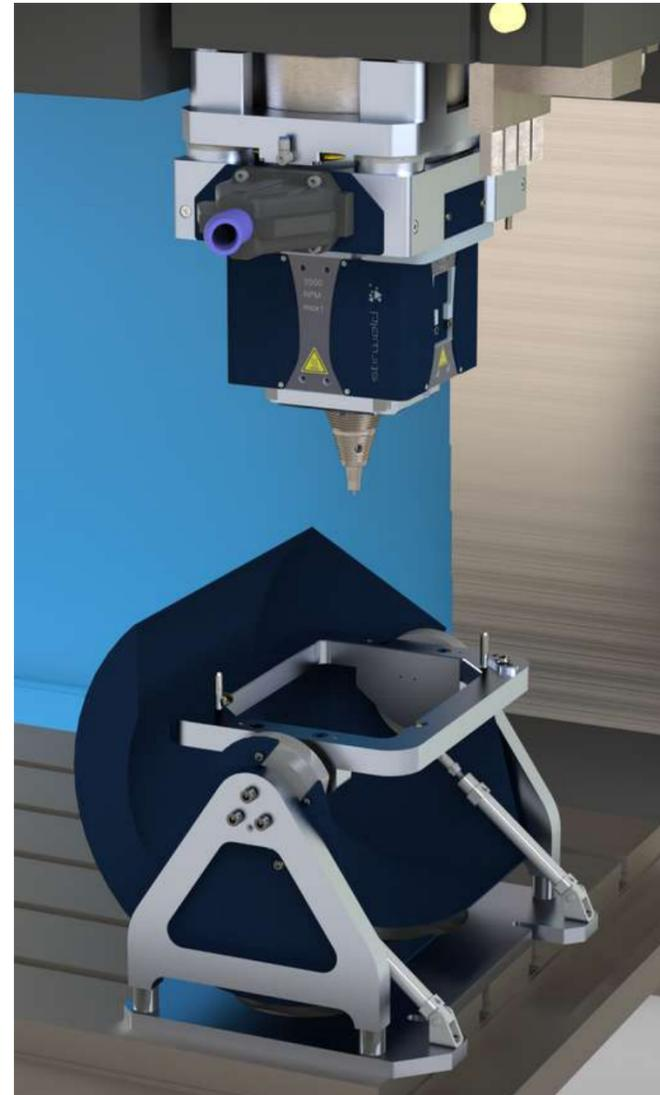
2 CNC spindle takes FSW head (automatic clamping device) the CNC table
